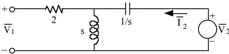
$$h_{12} = \left. \frac{\bar{V}_1}{\bar{V}_2} \right|_{\bar{I}_1=0}$$
