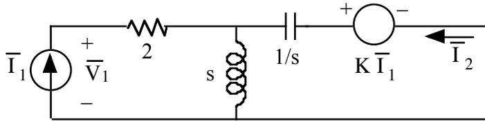
$$h_{11} = \left. \frac{\bar{V}_1}{\bar{I}_1} \right|_{\bar{V}_2=0}$$
