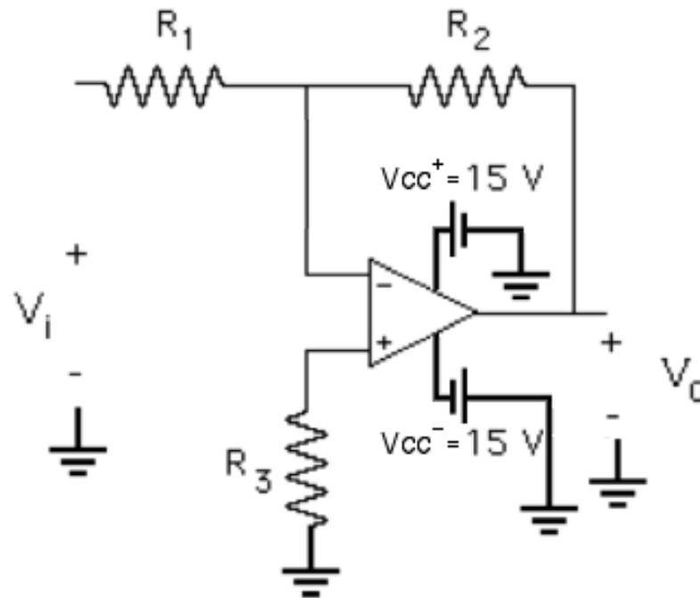
$$R_3 = R_1 \parallel R_2$$
